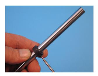
Two additional silver grub screws M3x4 081 need to be fitted into the collar ring and tightened, Use Loctite
