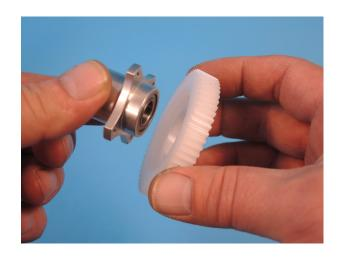
Four countersunk screws M3x8 025 are fitted loosely at first and then tightened in a cross pattern(3,9,12,6 o'clock). Use Loctite.
