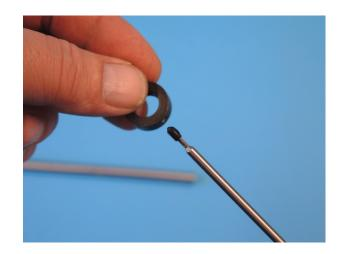
There is a small positioning hole in the mainshaft that must align with the tip of the grub screw. When the tip is in line with the hole tighten the screw.
