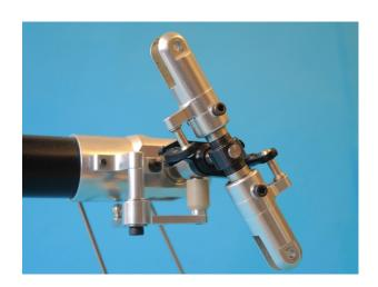
The rudder fin S870a and the elevator fin S870b are attached with two clamps H43 each and hex screws D197, large M3 washers 004 and lock nuts M3 008 onto the tailboom.
