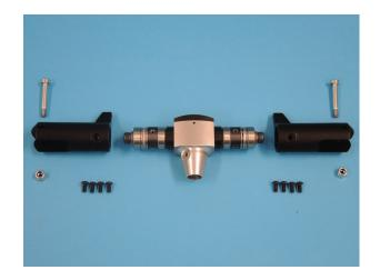
Push the blade grips onto the mounting ring and align the four holes. If the blade grips are tight, warm them up with a hair dryer. Fit 4 hex lens screws M3x6 D199 and shim washer 3x6x0,2 455 and mount them loosely with Loctite. Before tightening pull both blade grips with force outwards to eliminate endplay. This can be done by fitting the blade bolts and looping a rope through them to create the required pulling force. When done tighten the 4 screws on each blade holder.
