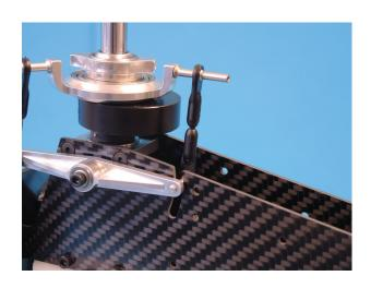
The swash plate holder H34 is provisionally fitted with two hex screws M3x35 D338 and lock nuts M3.
