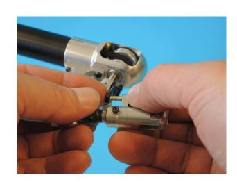
If a ball link is too tight then gently squeeze with a pair of pliers on the outside of the link until free movement is achieved. This can be repeated several times until the desired movement is achieved rather than one big squeeze and over doing the adjustment and ending up with a slack link.
