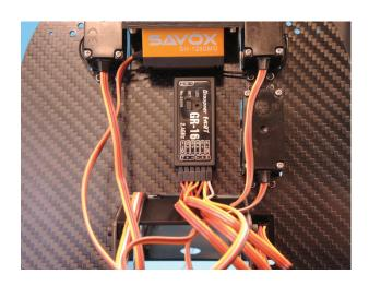
For a clean wiring installation fit a cable pad D342 on the left frame side as shown.
