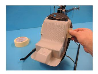
Now drill a hole with a 2mm drill in the lower left edge. Run the drill very slowly and watch for the drill coming through in the correct position in the seat. This hole is very important, if this is not drilled in the correct place all the other mounting holes will be wrong.
