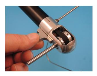
The rear end of the holder is attached with a lens screw M3x6 D199 and Loctite on the thread.
