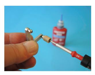
Fix the tail pulley on the tailshaft using two grub screws M3x5 0737 and Loctite. Take care that one grub screw is on the flat spot of the shaft and tighten first, Before tightening the second screw check that the shaft is level with the end of the bearing.
