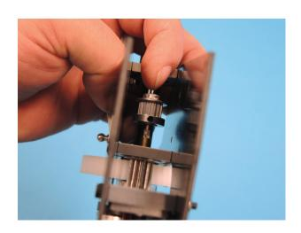
Tighten the belt wheel. Take care that the grub screw is really on the flat spot. Therefore leave the screw slightly loose and feel the endpoints of the flat spot while turning the motor back and forth slightly. When this is achieved tighten the screw.
