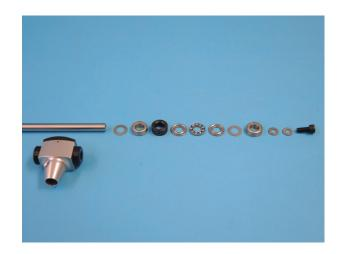
Push the feathering spindle D536 through the plastic bushes of the rotor hub D553 and adjust so it is centred.
