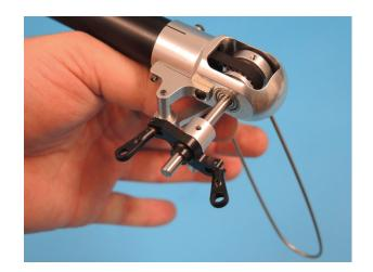
Now push one ball link onto the ball of a tail blade grip and check for bind free movement.
