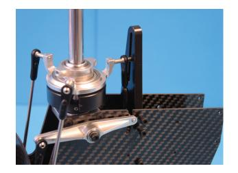
Overview of components of the rotorhub and feathering spindle.
