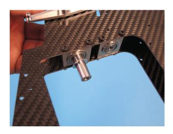
Fit the main gear assembly and check the clearance of the unit. The mainshaft must protrude a small distance from the bottom of the unit. If the clearance is too large then add washers 10x16x0.1 046 or 0.2 033. If the clearance is too small then add washers 5x10x0.1 044.
