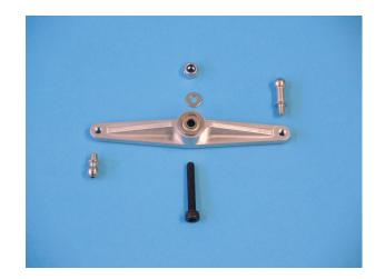
The ball link bolt M3x9 078 is attached to the flat side of the bellcrank S956 with Loctite. The ball link bolt M3x4 076 is attached to the opposite side with the ribbed flange using Loctite.
