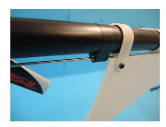
Screw two ball links S996 onto the tailrod. Make sure the the tailrod is fully screwed in with no threads showing especially at the rear end as vibration can fracture the rod.
