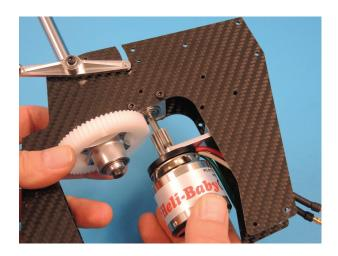
The holes in the frame should align with the holes of the motor carrier without being forced. Otherwise adjust the height of the pinion or add washers.
