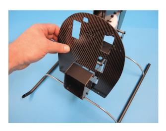
Add the tailservo holder H27. You may have to file the corners of the slot in the rear plate, but only a small amount. The holder should fit in the plate snugly. As soon as the holder fits into the slot (note it is slightly angled) as shown in the picture it should be secured with two hex screws M3x10 D328 on the mounting block H25. For this a ball wrench is useful but not essential.
