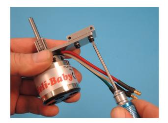
The motor unit is pushed from below into the upper frame.
