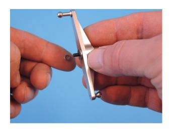
Attach the bell crank assembly through the hole in the left side frame and tighten using lock nut M3 008. An open spanner #707 is recommended to hold the nut.
