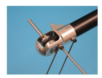
Two ball links 385 are screwed on the tailslider H52. Then slide the unit on to the tailrotor shaft and check for smooth movement on the shaft.
