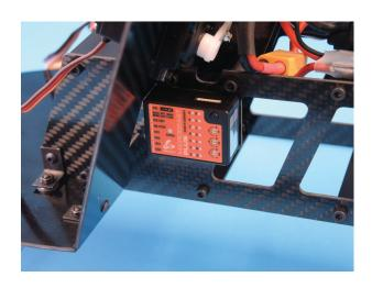
View of the wiring slot in the rear frame and the sockets of the Microbeast.
