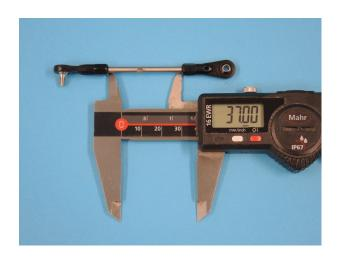
Fully screw in the 52mm H37 rod into the SRC arm H36 with Loctite, so that no thread is visable outside the unit (this is to avoid the risk of breakage in the threaded area). On the other end add a ball link with bolt D324. This rod has standard threads (clockwise turning).
