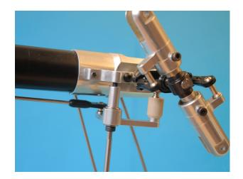
Check that the tail control rod is right angles to the tail bell crank and the servo arm, if not adjust the link at the servo until this is achieved.
