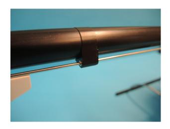
The distance between the rear of the rear block to the front edge of the tail rotor housing is 80mm.
