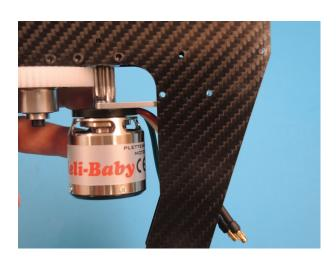
Tighten the assembly with two hex screws M3x35 D338 and lock nuts M3 008.
