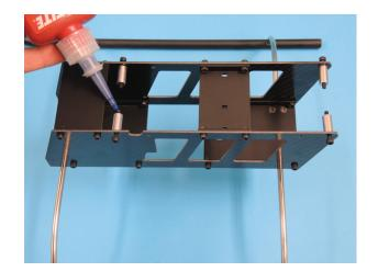
Next pull the hex screws out so they just dissapear into the connectors.
