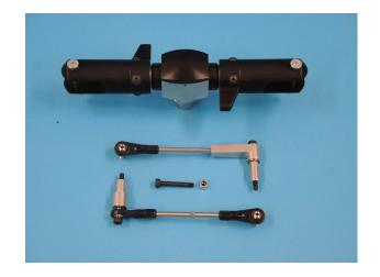
For mounting of the head, it is recommended to add a drop of oil into the shaft hole of the hub. Carefully push the head onto the shaft straight down, never turn the hub on the shaft (risk of seizing). When the bolt holes are aligned fit the jesus bolt D538 and tighten with a lock nut M3 008.
