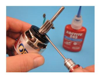
1. Fit the second grub screw M4x4 573 with Loctite and screw into the second hole of the pinion and tighten (1.7Nm).
