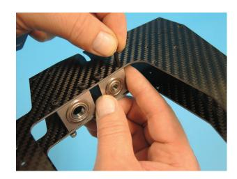
For a perfect fit of the three bearing blocks, press the two mainshaft bearings downwards/upwards during tightening of the screws. When all screws are tightened check the alignment of the frame edges, especially the lower edges.
