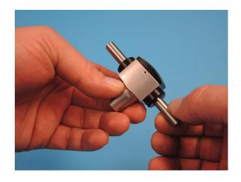
Now assemble all parts as shown in the picture. The inner washer is 0.5mm thick, the outer washer is 0.2mm. Lightly tighten the spindle screws M5 D568 to check clearance of the bearings. If the end play is too large, then add one 0.1mm washer to the 0.2mm shim. If it too tight then replace the 0.2mm shim with a 0.1mm shim. When clearance is correct there will be a small amount of movement and the bearings will turn freely, now tighten the spindle screws with Loctite.
