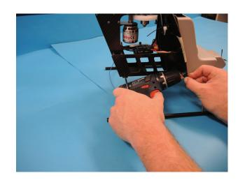
... and fix the seat with another slot screw and nut.
