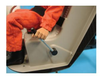
To mount the pilot use the elastic strip supplied in the kit. First, the band should be fitted flat over the seat without the pilot. Depending on which pilot is used a trial fitting is necessary. When happy, the elastic strip can be sewn together at the back of the seat.
