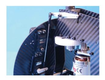
Attach the swash plate leveller D529 with the small recess to the top.
