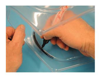
View of the completed canopy. Filling in the frame takes 30-40 minutes.
