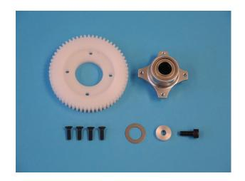
Press the freewheel unit H08 into the centre part of the main wheel H07 and take care that the holes in both parts are lined up.
