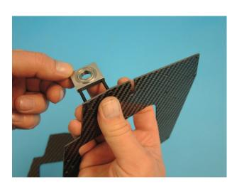
Put the motor shaft bearing block H04 between the frames and secure it with two screws M3x35 D338 and loosely fit lock nuts M3 008.
