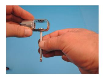
Push the tailrotor housing onto the tailboom and pull the belt as shown through the housing. Next insert the pulley wheel D579 into the belt and push it into the housing. Check that the spacer is on the correct side (where the pulley flange is smaller). Finally push the tailrotor shaft completely through.
