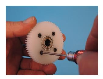
Push the prepared mainshaft assembly from above through the mainshaft bearings and from below fit a shim washer 0x16x0,5 757.
