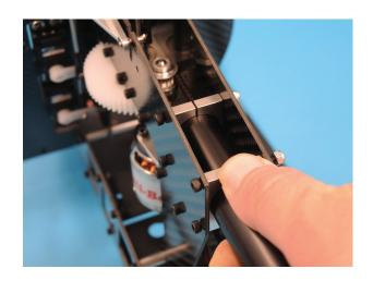
Tighten the lower two screws on the boom clamps and then tighten the belt by pulling the tailboom out.
