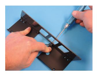
Mount the left lower side frame H13 in the same way with four hex screws M3x6 D196 und nuts M3 D547.
