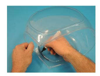
When the edges are fully blacked out, fill in between the lines to complete the canopy frame.
