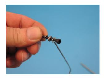
Now push the screw through the tail rotor housing.
