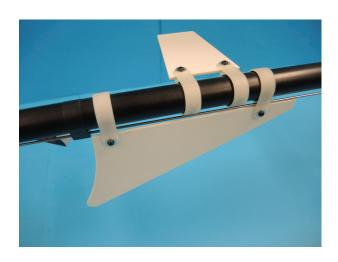
The tail control rod H49 is supported through two small mounts H46 and one large mount H45 at the front. Slide the wire through the three mounts. The distance of the front mount to the frame is 6-8mm. Use the supplied insulation tape to fix the mounts to the tail boom. It is important that the wire is mounted as straight as possible to prevent binding.
