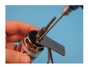
Fit two washers 002 onto hex screws M3x10 D328, fit them from below into the motor carrier and add Loctite to the threads.
