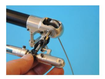
Tighten the tail rotor with a grub screw M4x5 035 locating it on the flat spot of the tail rotor shaft, apply Loctite to the screw.
