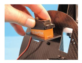
For easy mounting of the tailrotor servo use small pliers to hold the M2 lock nuts and after nut is in place use a 4mm open end spanner to tighten.
