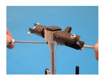
The rod with two ball links is attached to the blade grip with a hex screw M3x30 D337 and the stepped bush D540 using Loctite.
