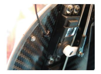
Now place the P-clip D348 on the left front hole of the receiver plate as shown, with hex screw M3x8 D197 and a large washer M3 004
