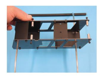
Push two inner connectors H22 between the outer ends of the upper frame. Then slide the upper frame between the connectors of the lower frame so that the screws are in line and push the hex screws into the holes. Do not tighten the screws at this stage.
