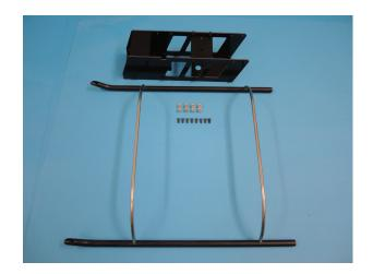
Attach four countersunk screws M3x8 025 to the front and rear bottom U-profile and Loctite each thread.
