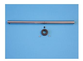
Screw a black grub screw with pointed tip M3x4 D314 in the hole in the collar ring H06. Use Loctite.
