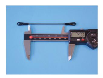
The rear elevator linkage is made from a grub screw M2.5x12 520 and two ball links 2.5 041. Mount the ball links as shown so that the swashplate is horizontal in neutral position. Usually the rod will have approximately 1mm free space between the links.
