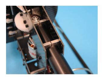
Push four hex screws M3x35 D338 through the clamps and fit four lock nuts M3 008. Do not tighten at this stage.
