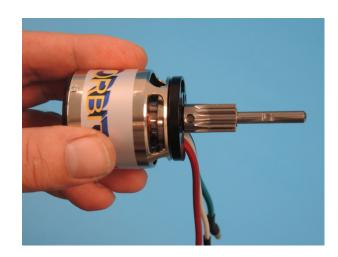
Then put some Loctite on the thread of the grub screw M4x4 573 and screw it into the pinion. Check before tightening that you are really on the flat spot. Therefore leave the screw slightly loose and feel the endpoints of the flat spot while turning the pinion back and forth on the shaft. When this is achieved tighten the screw with 1.7 Nm torque.
