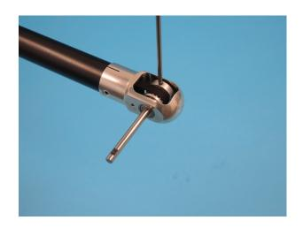
Bend the tail protection wire S868 over a one inch round bar and to an angle of about 150 degrees. Before bending the wire make sure that the eyelets are in line with the bend so that there are no alignment problems when fitted later. Fit the wire over hex screw M3x35 D338 with washer M3 002 under the screw head and shim washer 3x6x0,5 D312 on the other side of the eyelet.
