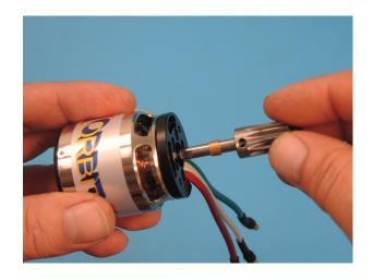
The grub screw hole in the pinion is positioned so that it lines up with the flat spot on the motor shaft.
