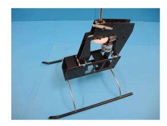
Overview of the rear canopy plate mount and the tail servo mount components.
