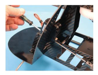
The tail servo with mounting screws, nuts and washers
