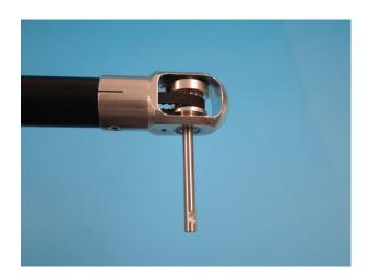
Remove the swashplate holder to fit the belt over the front pulley. This is possible without removing the holder, but easier with it removed. Place the two tailboom clamps with the cut slot uppermost. Make sure that the belt is turned a 1/4 turn the correct way, so that when the motor is turned anti clockwise the tail blade at the front side of the disk moves up towards the rotor disk.
