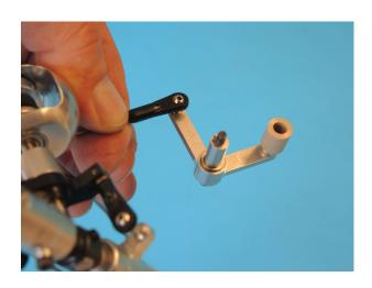
Screw the bellcrank with Loctite onto the holder. Make sure that the slider ball is located in the ball housing before tightening.
