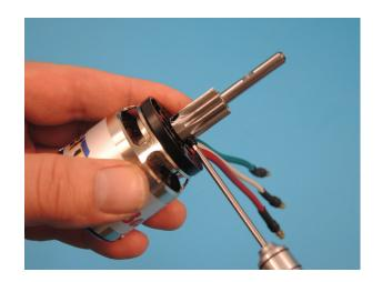
Put two washers 3x6x1 051 onto the hex screws M3x8 D197 and fit through the motor carrier H10. Finally add Loctite to the screws.
