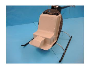
To fit the pilots seat belt, drill a series of 2.5mm holes in a row and then use a flat needle file to join the holes into a slot.
