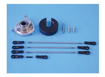
Screw two balls M3x9 078 and a guidance ball bolt D530 with Loctite into the outer ring of the swashplate D528.
