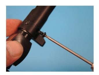
Assemble the left and right roll rods H35 with a large ball link D72 and a ball link with bolt D324. The ball link with ball is placed on the end with the left hand thread (with turned ring). When fitted, the length can be adjusted by turning the rod clockwise to reduce the blade angle and counter clockwise to increase blade angle.
