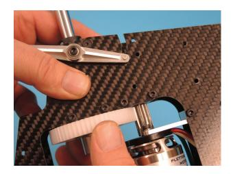
Push brass bush S988 onto the end of the motor shaft
