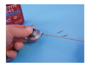
Assemble the elevator rod 106mm H33 with two ball links 2.5 041. The length between the links is 88mm.
