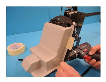
Screw the seat to the rear plate with a slotted screw D343 and a nut M2 S010 by hand without Loctite.
